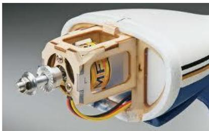
The **inrunner** has the mounting holes up front so the motor is behind the firewall.
