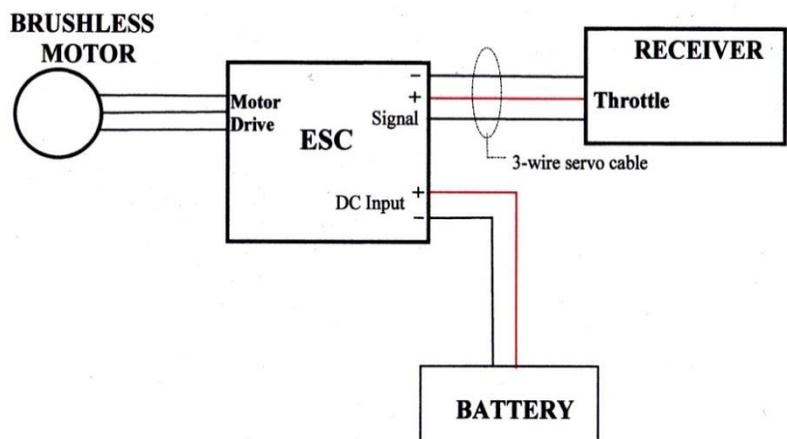
The third set of leads are the **battery** connections, which connects to the battery (makes sense) in which the positive lead is red and the negative lead black and **MUST** match the same colors as the battery leads. Later there are circuit diagrams showing actually “hook ups” including the type of connectors used.
