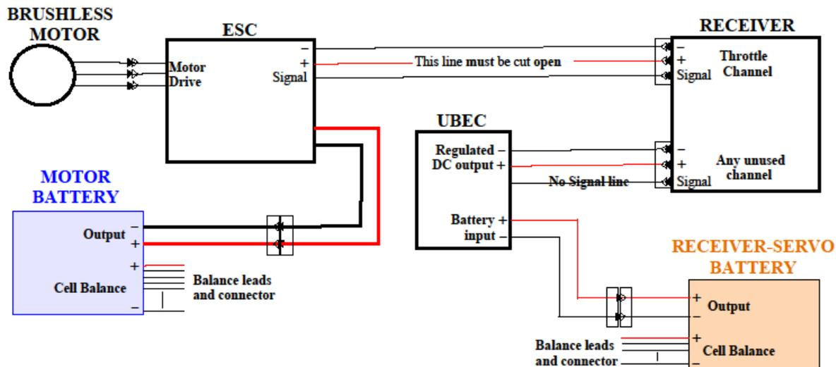
This circuit uses a **high current high voltage battery** for just the **motor** and a **smaller battery** for the **receiver** and **servos**
