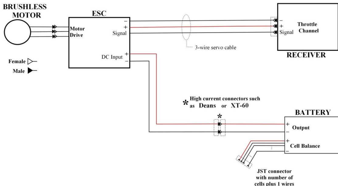
**ESC: Electronic Speed Controller** - In this system, the ESC may have a Battery Eliminator Circuit (BEC) but it is not used and the positive wire (usually Red) must be cut open
